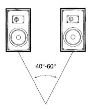
Harbor JBL Series loudspeakers are designed to produce a flat frequency response in the home when located free standing, at least 1 foot from a wall.
